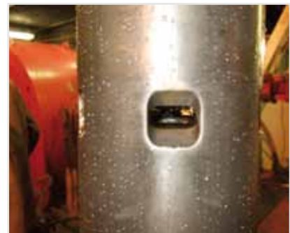
Open circulating ports provide generous flow area
