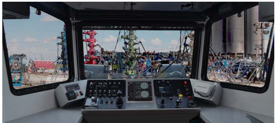
The wide angle of view in the control cabin improves safety and coordination with fracturing and wireline operations.
