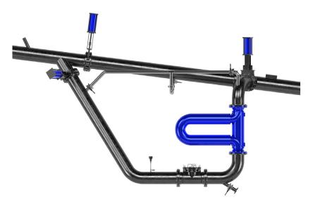
The FLAGHD service flowmetering sensor delivers an outflow signature three times faster than the conventional flow check method. Instead of a 15-minute flow check, an outflow signature is accomplished in just 5 minutes for each pump stop.
